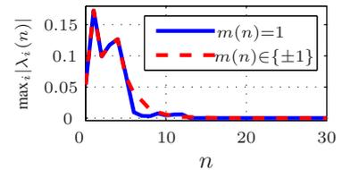
**Fig. 2.** Maximum absolute value of the eigenvalues of  $[\mathbf{A}_r(n) - \mathbf{A}_t(n)]$  along the iterations; Ikeda map ( $\mathbf{x}(0) = \mathbf{0}$ ;  $\hat{\mathbf{x}}(0) = [0.1 \ -0.1]^T$ ;  $C_1 = 0.4$ ,  $C_2 = 0.9$ ,  $C_3 = 6$ , and  $R = 1$ ).
