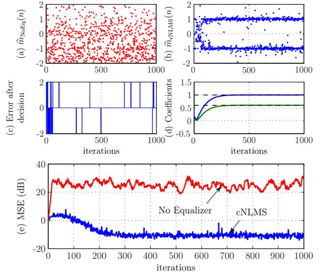
**Fig. 3.** Estimated sequence with (a) No equalizer and (b) cNLMS ( $\mu = 0.1$ ,  $\delta = 10^{-2}$ ,  $\varepsilon = 0.1$ ); (c) Errors after decision; (d) Average of the coefficients of cNLMS and Wiener (dashed lines); (e) Estimated cMSE; average of 1000 runs, SNR = 30 dB;  $M = 2$ ;  $\Delta = 0$ .
