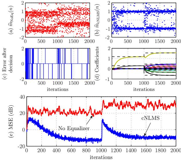
**Fig. 4.** Estimated sequence with (a) No equalizer and (b) cNLMS ( $\mu = 0.5$ ,  $\delta = 10^{-5}$ ,  $\varepsilon = 0.1$ ); (c) Errors after decision; (d) Average of the coefficients of cNLMS and Wiener (dashed lines); (e) Estimated cMSE; average of 1000 runs, SNR = 30 dB;  $M = 15$ ;  $\Delta = 8$ .
