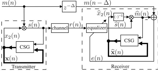
**Fig. 1.** Chaotic communication system with an adaptive equalizer.
