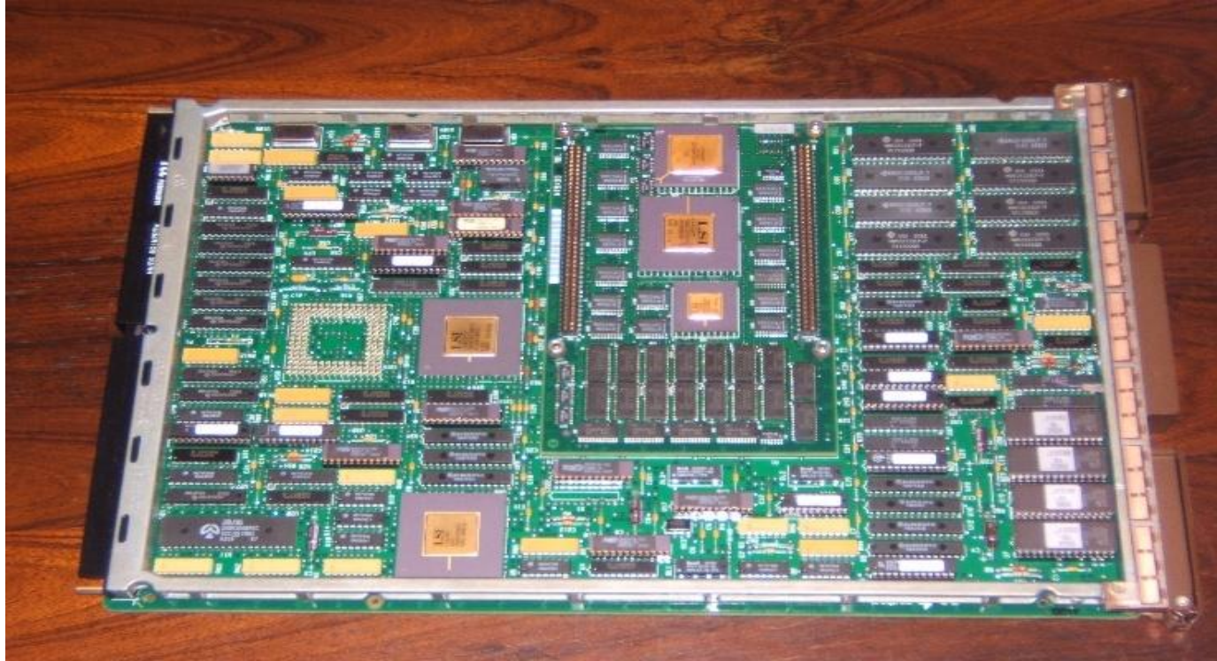
CPU p/ Estação radio-base Northern Telecom (1993)
