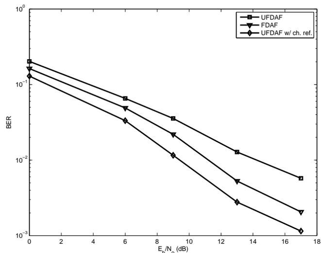
**Fig. 6.** BER for time-varying channel with  $fdNT_c = 0.0002$ , paths with relative delay equal to 0,  $2T_c$ ,  $6T_c$ ,  $9T_c$  and  $12T_c$  and respective relative powers of 0dB, -1dB, -3dB, -6dB and -9dB.
