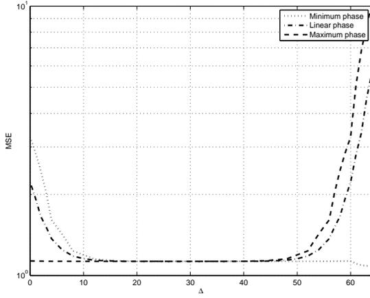
**Fig. 3.** MSE as a function of the position of the FFT window of the UFDAF and  $\sigma_x^2/\sigma_n^2=20\text{dB}$ .
