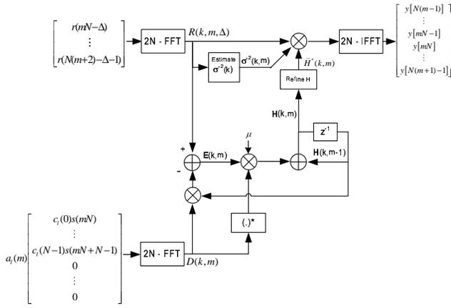
**Fig. 2.** Enhanced UFDAF equalization technique
