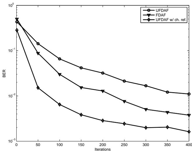
**Fig. 5.** Time to convergence measured in terms of BER for a three-path Rayleigh block fading channel with relative delay 0,  $4T_c$  and  $12T_c$  and respective relative powers of 0dB, -3dB and -6dB.
