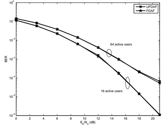
**Fig. 4.** Bit error rate for 64 and 16 users for a block Rayleigh fading channel with relative delay  $0, 2T_c, 6T_c, 9T_c$  and  $12T_c$  and respective powers of 0dB, -1dB, -3dB, -6dB, -9dB.
