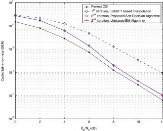
Figure 5: The BER performance of coded OFDM system
